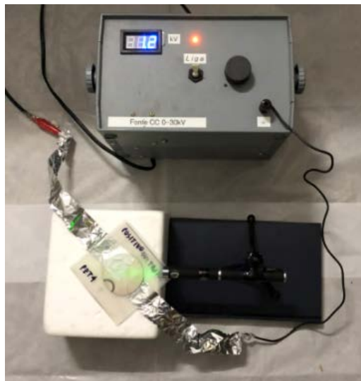
Figure 1. The experimental setup performed inside the building (indoor) with 47 m laser beam length. It is shown the high voltage power supply (grey box) where the PZT4 ceramic disc covered by thin layers of acetate is connected by strips of aluminum. The disc is supported by the white styrofoam box. The laser pointer supported by a tripod has continuous activation.
