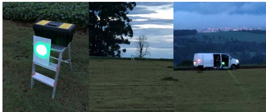
Figure 3. The three photos show different views of the experimental setup used in the field (outdoor). The left photo shows the laser beam profile projected in the whiteboard with 1-centimeter grid. The middle photo shows the mentioned devices that are far 120 m from the laser pointer. The right photo shows the position of the laser pointer far 120 m from the whiteboard.
