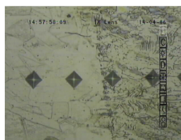
(c) micrograph of HAZ
