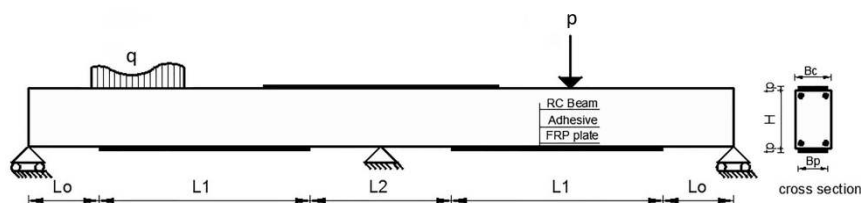
Figure 1. RC beam bonded with an FRP plate
