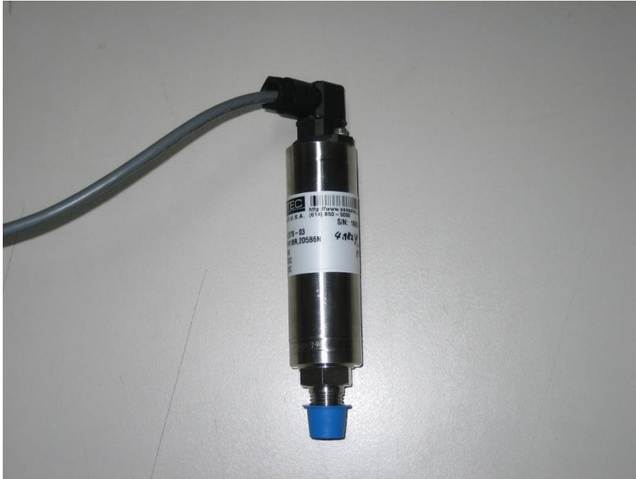
Fig. 3.8. Pressure sensor used in primary and exit flow (FPA).
