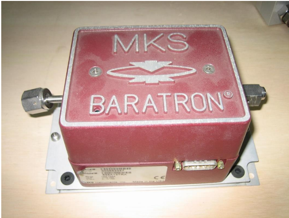
Fig. 3.9. Pressure sensor used in secondary flow (BARATRON 698A13TRA).
