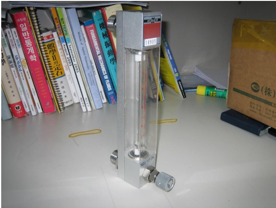
Fig. 3.6. Mass flow rate meter used in primary flow (GR112-1-A-PO).
