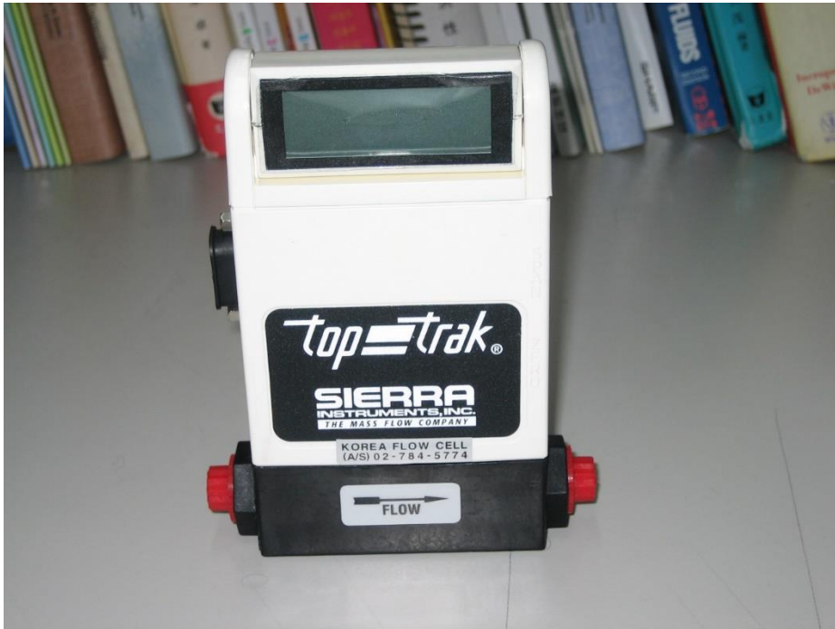
Fig. 3.7. Mass flow rate meter used in secondary flow (GR112-1-A-PO).
