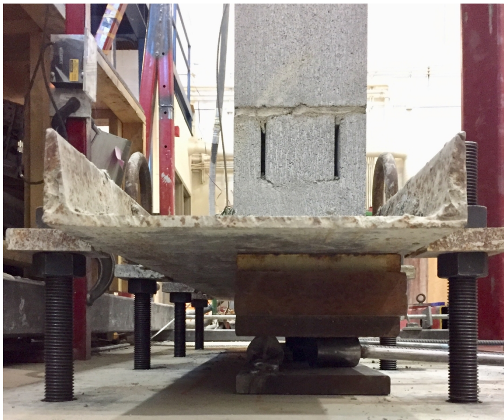
Figure 6: Vertical Section of Wall with Pinned-Fixed Supports (a) and Base Detail Showing the Wall Placed Eccentrically in the C-channel and the Steel Beneath (b)
