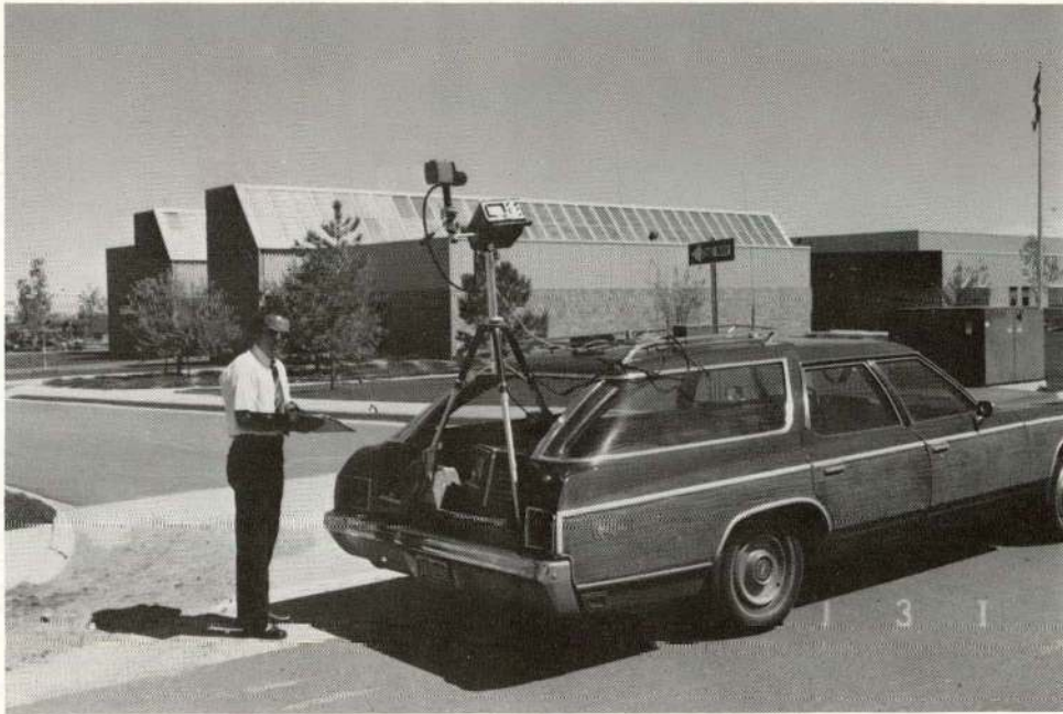
Figure 2-1. Ground-Based Thermographic Equipment
