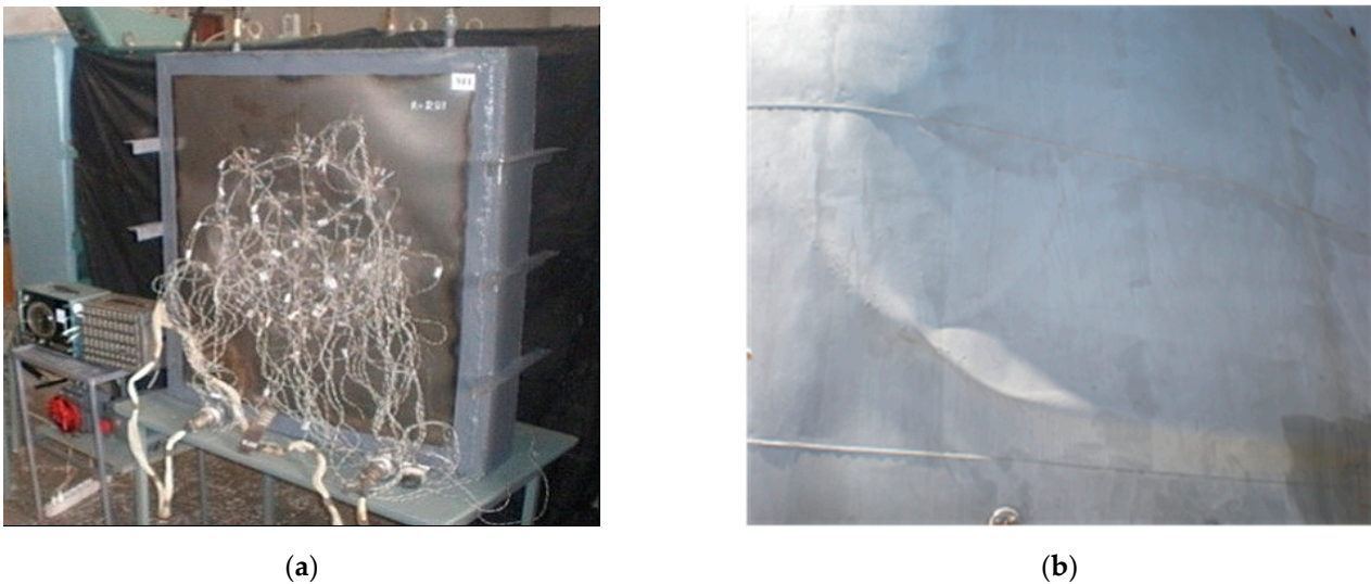
Figure 1. View of the dent on the model (a) and full-scale object (b) [33,34].
