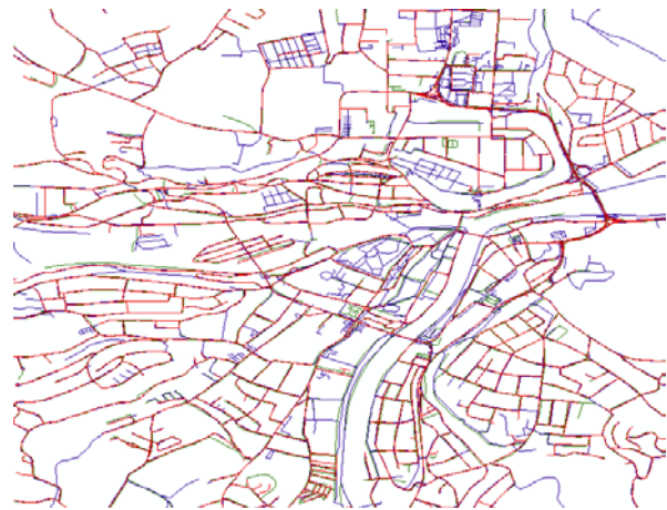
Figure 4: City of Steyr with representations of OSM (blue), GIP (green) and TomTom (red)
