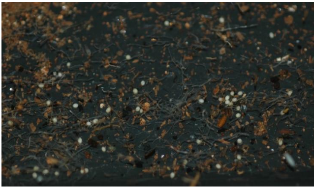
Figure A3-5: Materials from the bottom sieve are spread out on a black plate and white cysts are counted. The root system is also examined for any white cysts remaining on the roots
