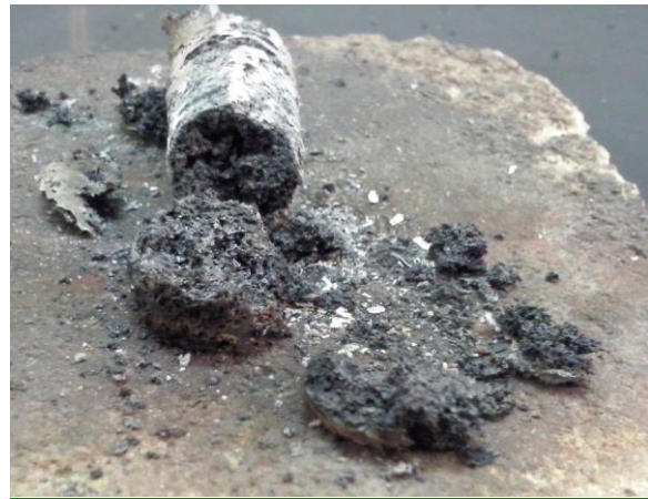
Figure 6. Solid residues left after burn test of Al/BADGE17 burn test.
