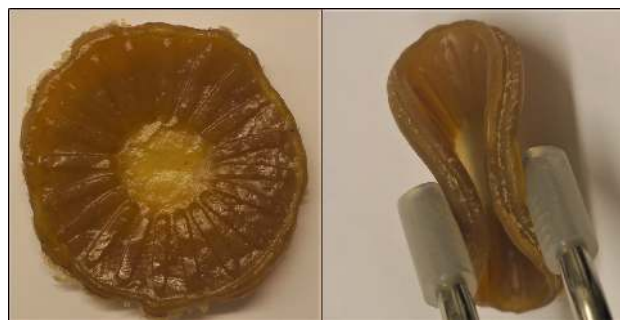
Figure 4: Elasticity of the plasticized soy protein after measurement, visualized by manual deformation. The deformation is completely reversible.
