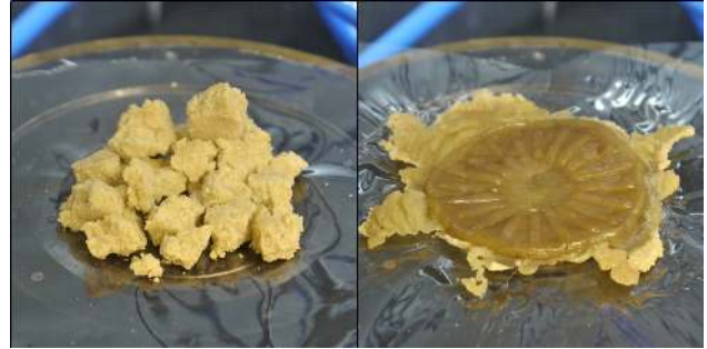
Figure 2: Soy protein matrix with a moisture content of 51.7% before (left) and after (right) measurement in the closed cavity rheometer.
