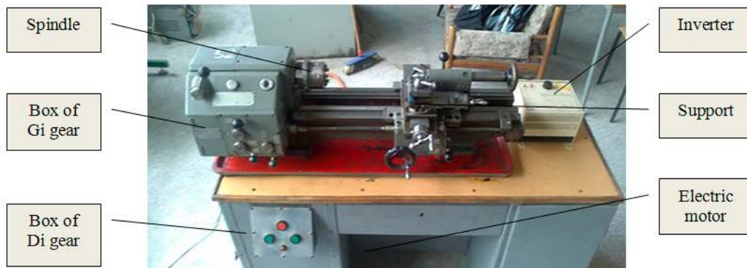
Figure 2. View of a TSB16 lathe with inverter.
