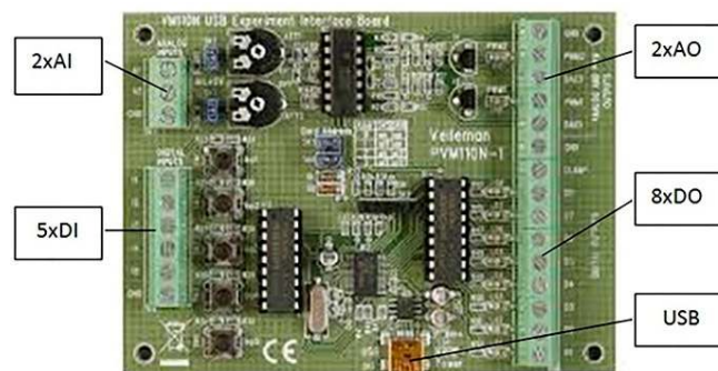
Figure 7. Velleman K8055 interface.
