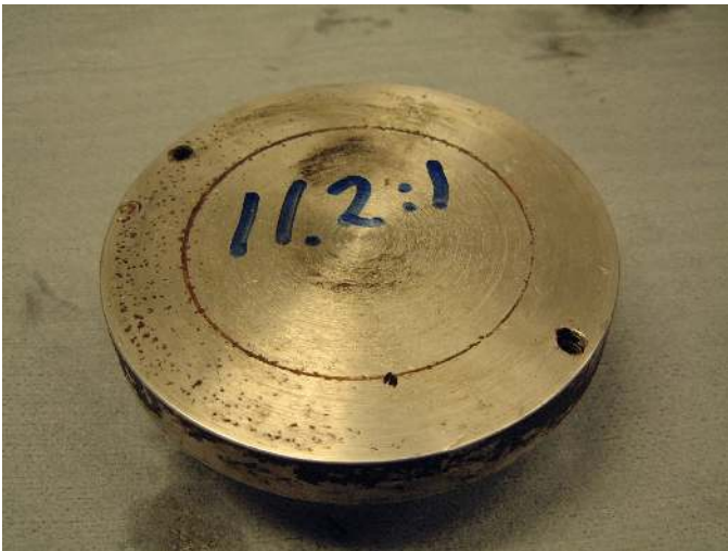
Figure 5. Flat piston crown used in the disc geometry.
