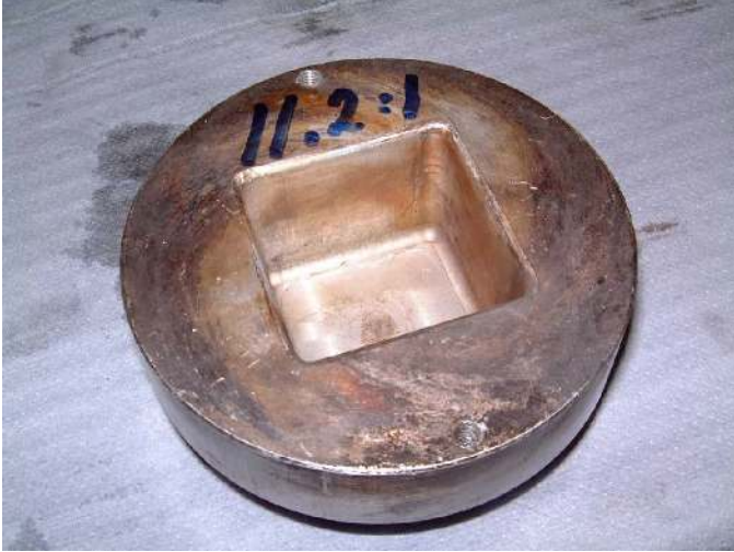
Figure 3. Piston crown with square bowl combustion chamber.
