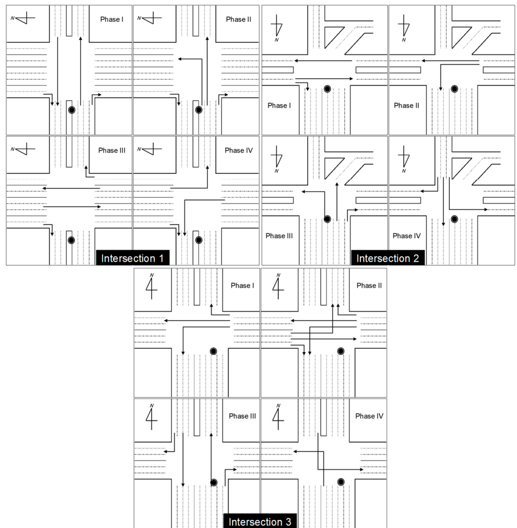
Figure 2. Traffic flow in each of four green light phases (phase I to phase IV) during traffic signal cycles and the measurement point at each intersection (black circles).
