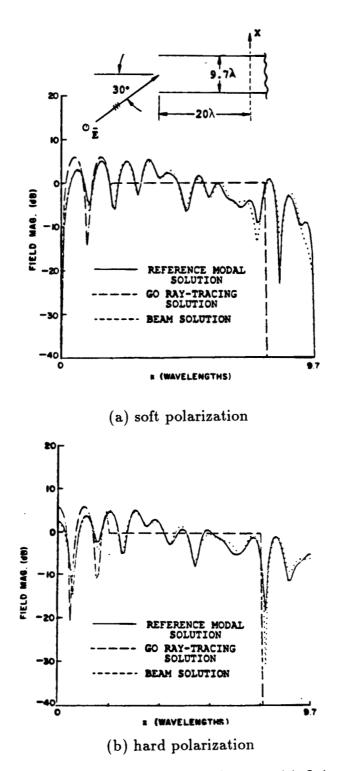
Figure 6.1: Fields at a cross-section inside a semi-infinite parallel plate waveguide illuminated by a plane wave
