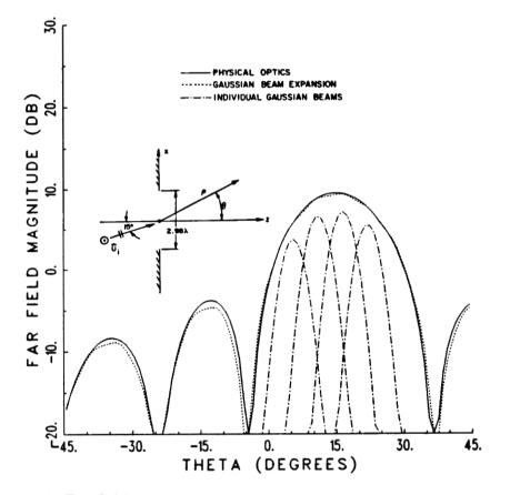
Figure 4.6: Far field pattern of a sub-aperture illuminated by a plane wave and 4 component Gaussian beams, 3.5 beams/lobe.  $\Delta \theta = 5.5^{\circ}$ ,  $b = 64.0 \lambda$ ,  $w_o = 9.0 \lambda$ .
