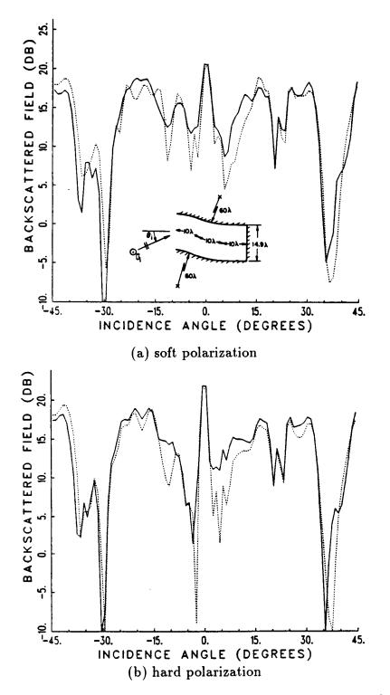
Figure 6.4: Backscatter from an open-ended 2-D S-shaped waveguide cavity with a planar termination, L/d = 2, 7 sub-apertures,  $\Delta \theta = 7.69^{\circ}$ . — hybrid modal solution, - - - GB solution.
