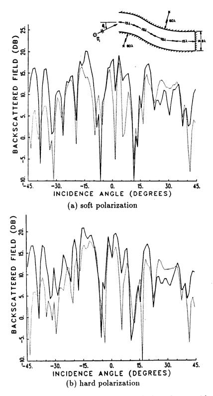
Figure 6.6: Backscatter from an open-ended 2-D S-shaped waveguide cavity with a planar termination, L/d = 4, 7 sub-apertures,  $\Delta \theta = 7.69^{\circ}$ . — hybrid modal solution, - - - GB solution.
