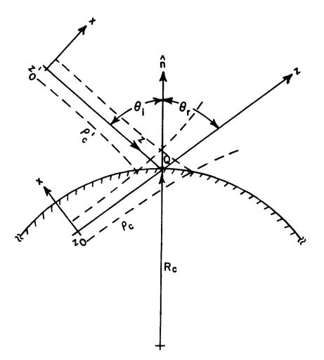
Figure 5.2: Gaussian beam reflecting off a curved surface.
