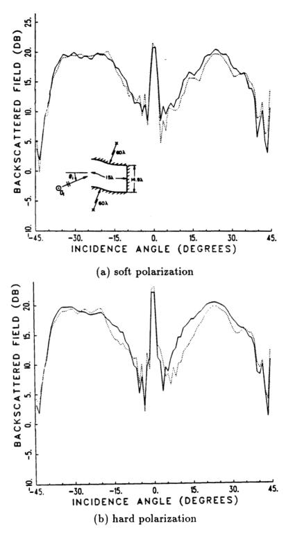
Figure 6.3: Backscatter from an open-ended 2-D S-shaped waveguide cavity with a planar termination, L/d = 1, 7 sub-apertures,  $\Delta \theta = 7.69^{\circ}$ . — hybrid modal solution, - - - GB solution.
