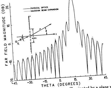
Figure 4.9: Far field pattern of an aperture illuminated by a plane wave. 5 sub-apertures, 4.5 beams/lobe,  $\Delta \theta = 4.3^{\circ}, b = 105.8 \lambda, w_o = 11.6 \lambda$ .
