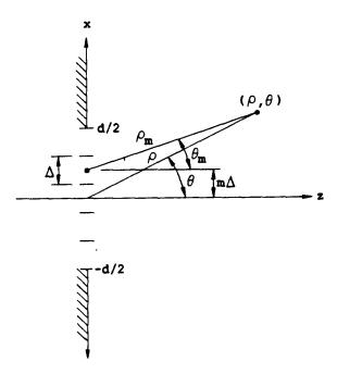
Figure A.2: Geometry of the  $m^{th}$  sub-aperture defining  $\rho_m$  and  $\theta_m$ .
