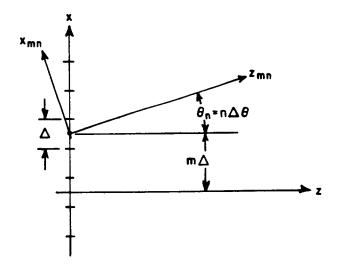
Figure 4.2: Coordinate system of the  $mn^{th}$  shifted, rotated Gaussian Beam.
