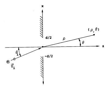
Figure 4.1: Plane wave incident on an aperture of width d.
