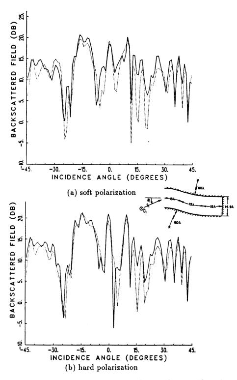
Figure 6.5: Backscatter from an open-ended 2-D S-shaped waveguide cavity with a planar termination, L/d = 3, 7 sub-apertures,  $\Delta \theta = 7.69^{\circ}$ . — hybrid modal solution, - - - GB solution.
