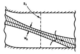
Figure 5.3: Gaussian beam crossing the plane of the termination inside a waveguide cavity, away from the walls.
