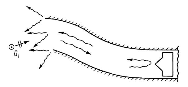
Figure 2.1: Scattering components of a 2-D open-ended waveguide cavity.
