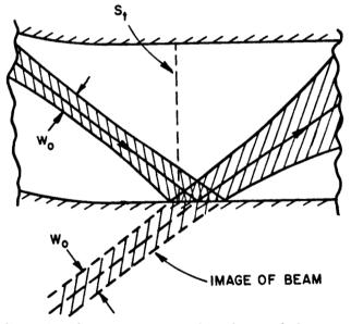
Figure 5.4: Gaussian beam crossing the plane of the termination inside a waveguide cavity, near a wall.
