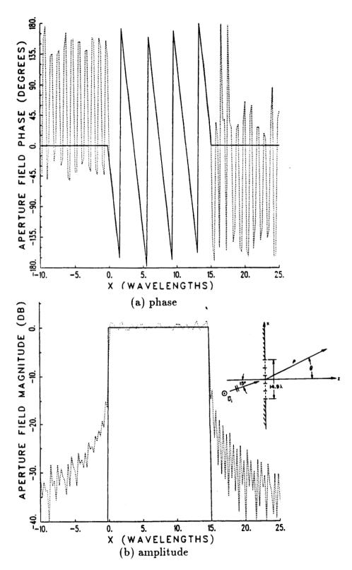
Figure 4.10: Fields in the plane of an aperture illuminated by a plane wave. 5 sub-apertures, 3.5 beams/lobe,  $b = 64.0 \lambda$ ,  $w_o = 9.0 \lambda$ .
