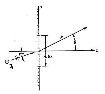
Figure 4.5: Aperture illuminated by a plane wave incident at 15° with 5 sub-apertures.
