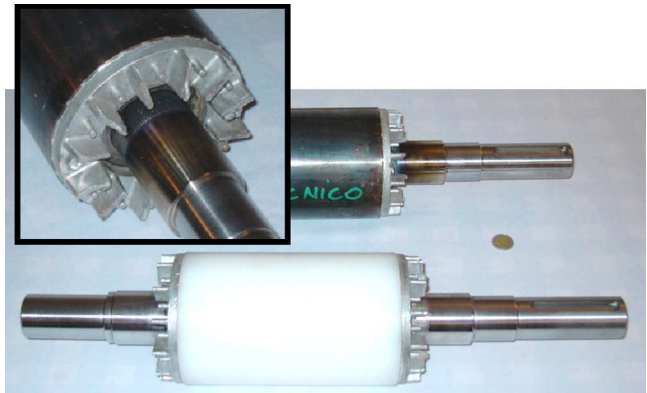
Fig. 2. Example of the original and “plastic” rotor (MA160 motor) with the short-circuit ring detail (for all the prototypes, there are 12 fins and tips on the ring).
