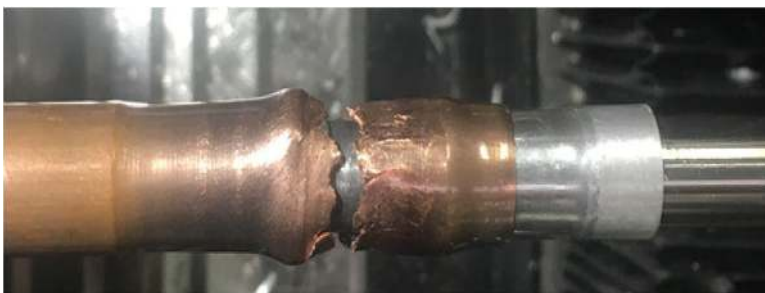
Fig. 14 Fracture of bimetal tube
