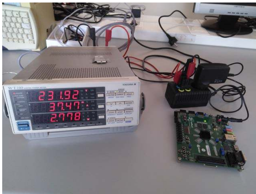
Fig. 6. Power measurement setup
