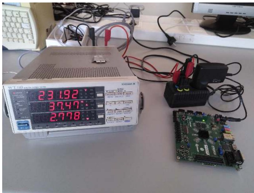
Fig. 6. Power measurement setup
