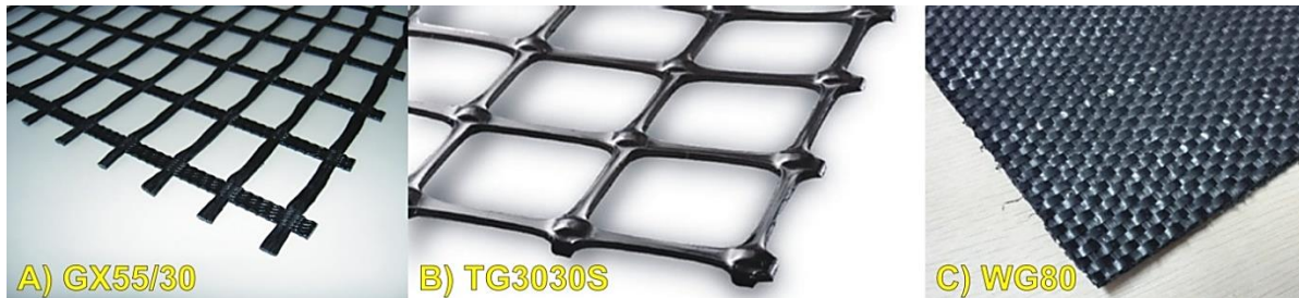
Fig. 2: Geosynthetic reinforcements used in the laboratory testing.
