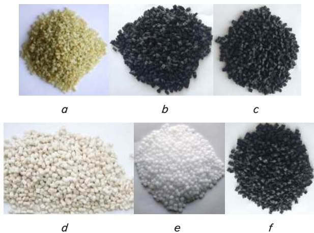
Fig. 1. Physical appearance of PCM granules selected for experimental research: a – Nylon 66; b – PA-6-210KS; c – PA6/6.6 R196-GF30; d – Kocetal GF705; e – Kocetal K300; f – UPA-6-30
