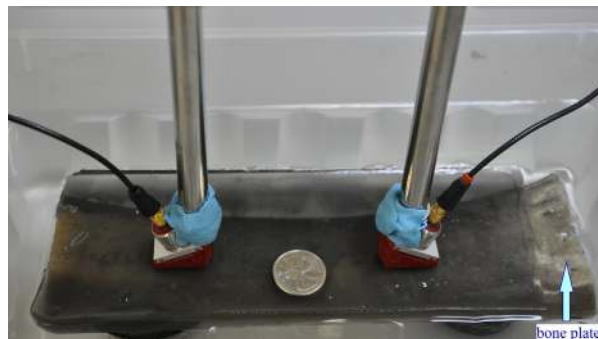
Fig. 1. The experimental setup for the bone plate (BP) and soft tissue/bone plate (STBP) measurements. Shown here is the STBP sample. Some soft-tissue material was scraped off at the end to show the bone plate. Water below the bone plate is used to mimic marrow. A Canadian 25-cent coin (23.8 mm in diameter) is used to show scale.
