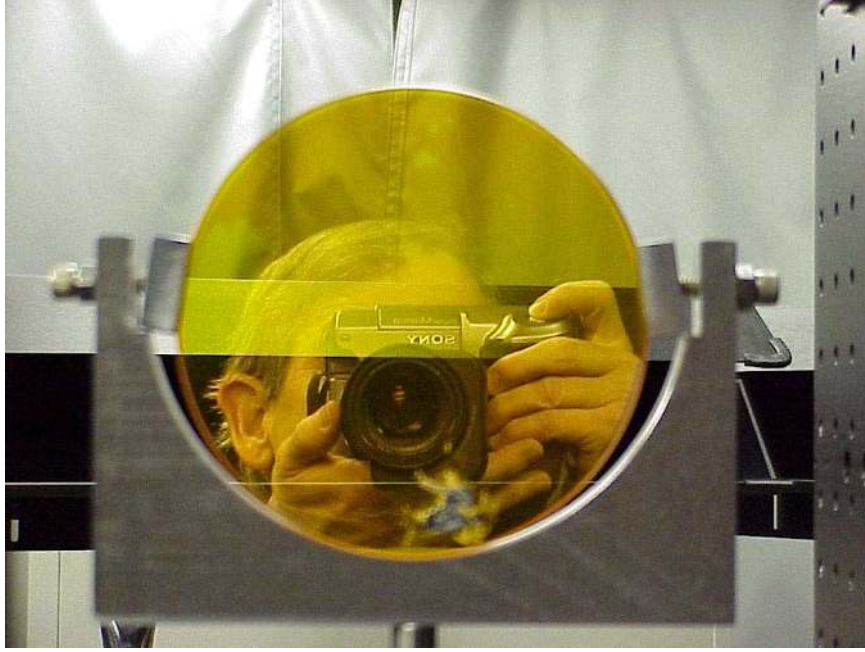
Figure 3.6: A photograph of the ZnSe window in its mount. The uneven coloring of the window is indication of regions where the ZnSe substrate is exposed because the AR coating flaked off.
