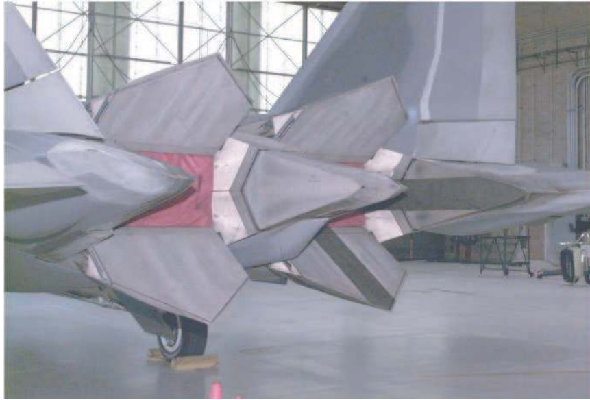
Figure 6.1: Rear view of the F/A-22. The stripe along the sidewall and lower divergent flap is a high-emittance, black paint used for deriving surface temperatures from in-flight radiometric measurements.
