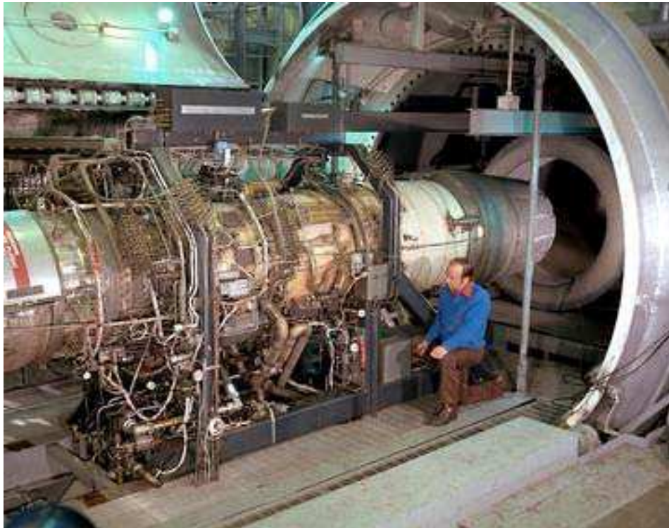
Figure 2.12: F100 engine in the altitude test cell at the Propulsion Systems Laboratory, NASA Glenn Research Center.
