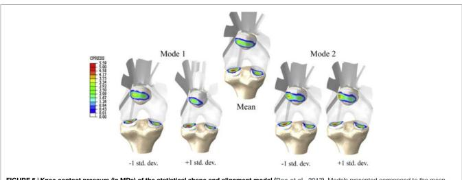
FIGURE 5 | Knee contact pressure (in MPa) of the statistical shape and alignment model (Rao et al., 2013). Models presented correspond to the mean shape and the variation of the first two modes between ±1 SD from the mean shape.
