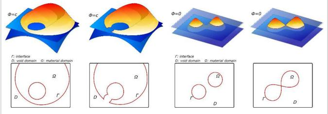
FIGURE 6 | Examples of level-set functions  $\phi$  and their corresponding material domain  $\Omega$  before and after the design update, adapted from Dijk et al. (2013).
