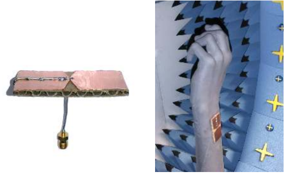
FIGURE 16. Antenna prototype with coaxial feeding bent around the loop (left) and the on-body measurement setup (right).
