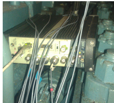
Fig. 3. Apparatus used for measurements B&K 3560-B-120
