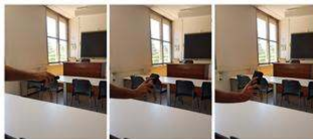
Fig. 3 Measures looking at the table (angle 0°), looking at the back of the chair in front (angle 30°) and looking at the end of the classroom (angle 60°) for the venue with windows facing south.
