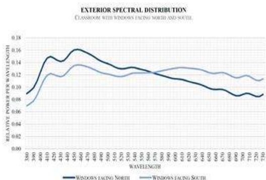
Fig. 6. Exterior spectral distributions. Classroom with windows facing north and south.
