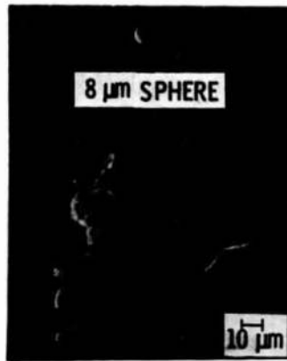
(a) STRING OF WEAR PARTICLES AND 8 micrometer DIAMETER SPHERE FROM 530-hour SAMPLE.
