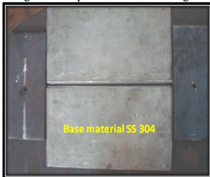
Fig.2 Specimen Is Tapered For Weld Strength
