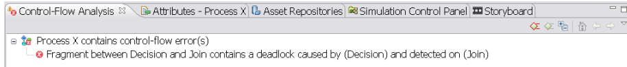
Figure 10: Example of an error message following the “caused by - detected on” pattern.
