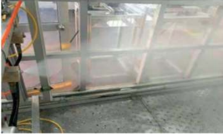
FIGURE 5: Atomization effect of 4 MPa pressure nozzle.
