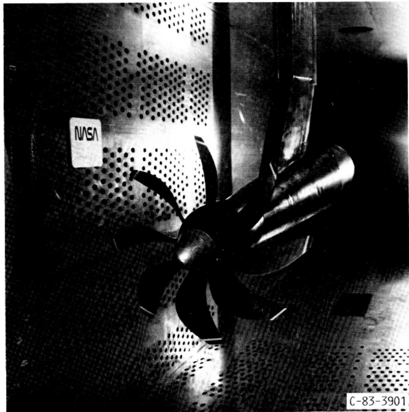
FIGURE 2.- SR3C-X2 PROPFAN MODEL WIND TUNNEL INSTALLATION.
