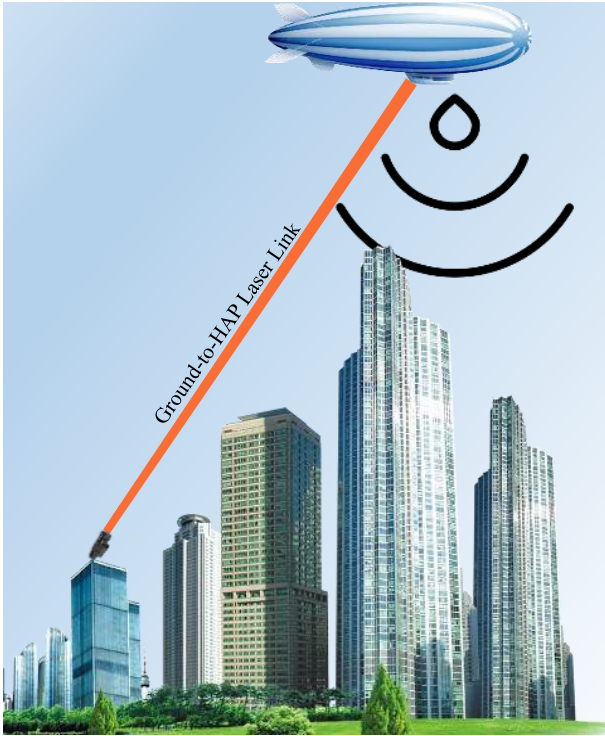
Fig. 1. A typical illustration of a HAP-based FSO communication link. HAPs are usually placed in the stratosphere layer where the thin air is relatively calm and the wind speed is low, and thus, the link length is commonly larger than 17 km [1].
