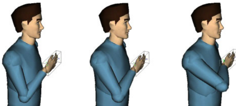
Figure 7. If collisions are detected (left) the orbit angle is updated and a valid posture is eventually found (center). As the hand gets closer to the body, the orbit angle is continuously updated (right).
