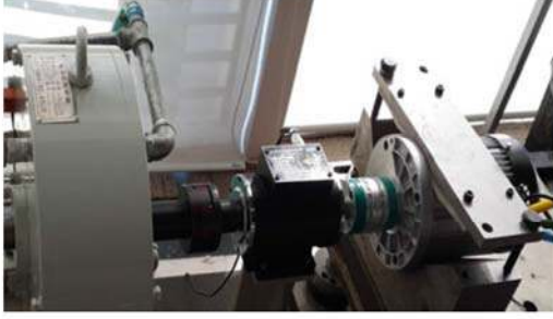
Fig. 2 Experimental step of the PMSM drive system.
