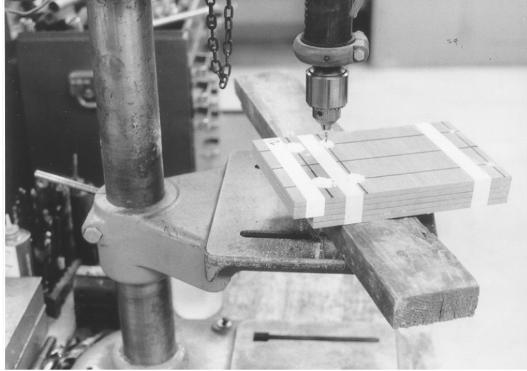
Fig. 2.2. Pre-drilling pilot holes in GFRP sheathing panels
