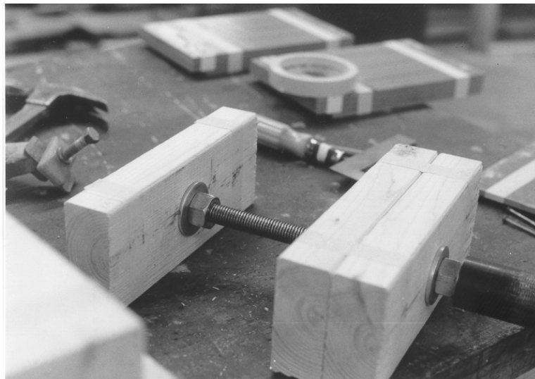
Fig. 2.3. Aligning loading holes in wood framing
