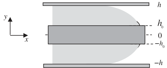
Fig. 11. Geometry for the yield stress fluids. The plug zone goes from -y_0 to y_0 . The channel width is 2h .
