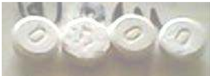
Figure A3. Picture of ELYS CHEMICALS (NAIROBI-KENYA) fake quinine tablets sample. Note: The picture was taken after the friability test.
