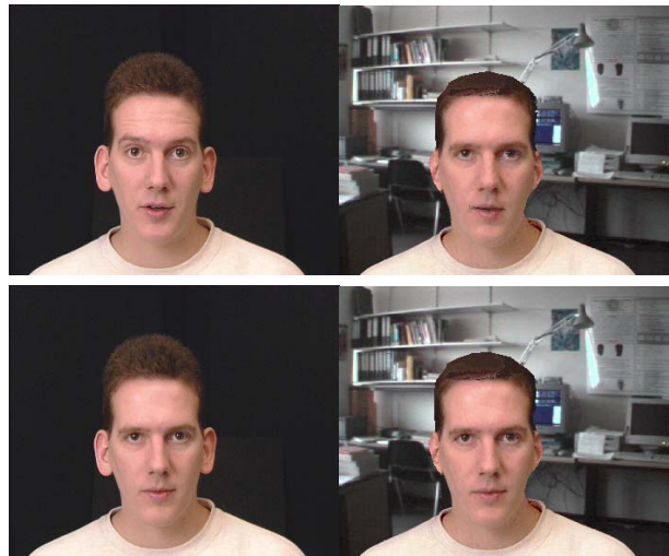
Figure 15: Camera frames (left) and corresponding reconstructed synthetic frames in a virtual environment(right).
