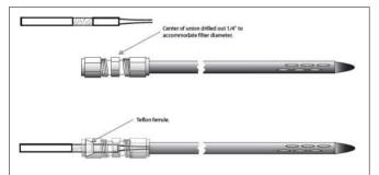
FIGURE 1 | Representation of soil probe design used to sample volatiles belowground. Probe is inserted into soil and connected to a vacuum pump. Reprint from "Extending explorations of belowground herbivore-induced plant volatiles: attracting natural enemies of root pests in multiple contexts (Ali et al., 2012).
