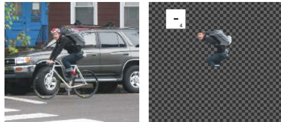
Figure 1. What’s moving ? Given an image with motion blur, we seek to infer the blur kernel and the region it affects. The image on the right shows a segmentation of the blurred object in the image, and an estimate of the blur kernel generated by our algorithm.
