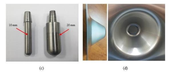
Figure 1. (a) Fixture and machine setup, (b) part dimensions and the investigated process parameters, (c) forming tools, and (d) final part.
