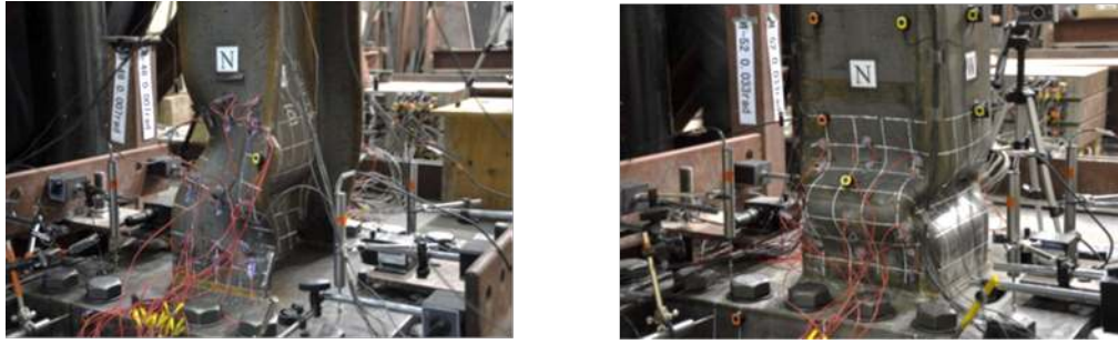
Figure 1. Residual column axial shortening of steel columns: (Left) W14x53 (axial shortening = 55 mm) and (Right) HSS 254x9.5 mm (axial shortening = 72 mm) (Images were retrieved from [7]).
