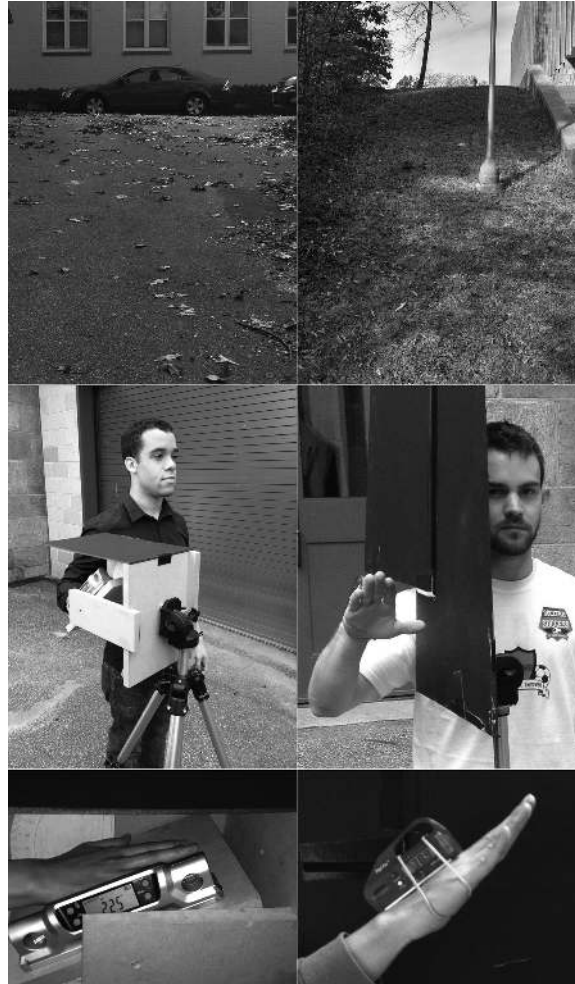
Figure 2. Hills used at SWAT (upper left; 6.3°) and at OSUM (upper right; 21.7°) are shown from the observers' viewpoint. Below are shown a palm board apparatus (middle left) with inclinometer (lower left) and a free hand apparatus (middle right) with inclinometer (lower right).
