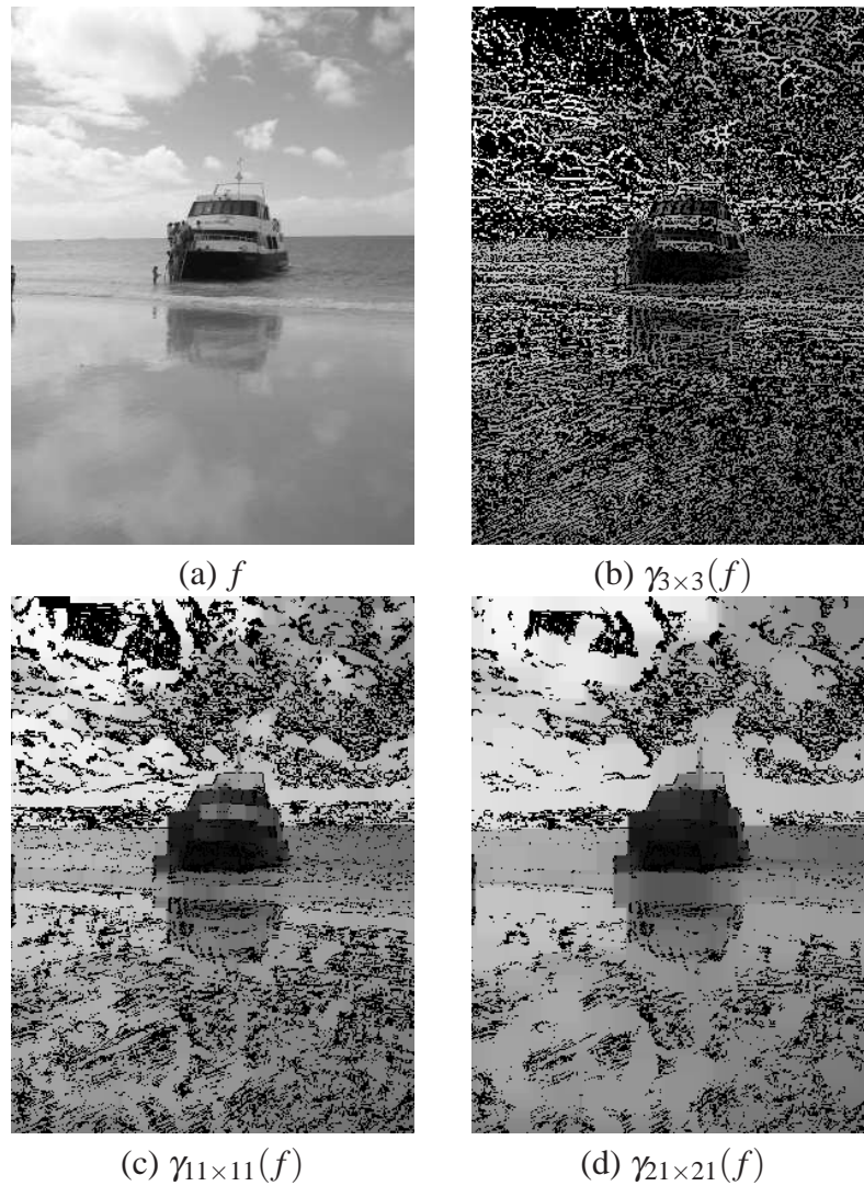
FIGURE 12. Density of opening anchors for increasing sizes of the structuring element. From left to right, and top to bottom: original (a) and openings with a squared structuring element B (of size 3 \times 3 , 11 \times 11 , and 21 \times 21 respectively).
