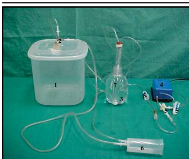
FIGURE 1 - The anesthetic equipment: (1) the induction chamber; (2) three way unidirectional key; (3) the glass cylinder partially filled with water containing the tube with the anesthetic drug; (4) the air compressing machine; (5) the y-shaped tube an two regulators; (6) the management plastic hood; (7) the laboratory tube with the needle.
