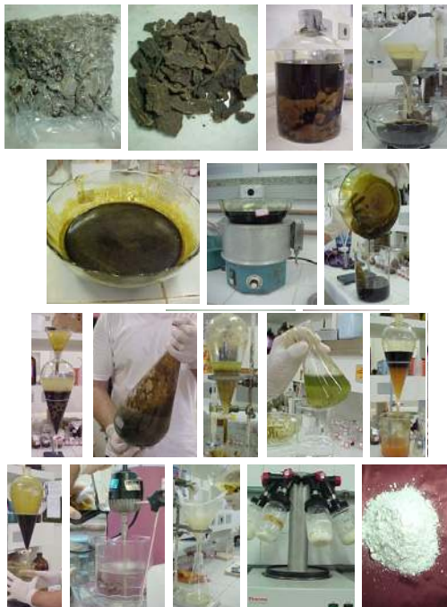
FIGURE 2 - Extraction of propolis (sequence of method of extraction of Water-Soluble Derivative of Propolis).
