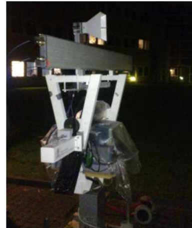
Fig. 2 Rotation rig with receiver antennas and spectrum analyzers
