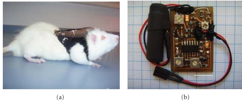
FIGURE 7: Chronic instrumentation of a freelymoving rat. (a) Rat with a portable stimulator in a backpack; (b) stimulator purchased from the company Rückmann and Arndt, Berlin, Germany. Scale bar in (b): 10 mm.
