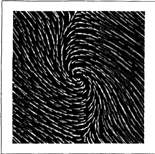
Figure 12: OLIC of a simple pendulum model with speed encoding
