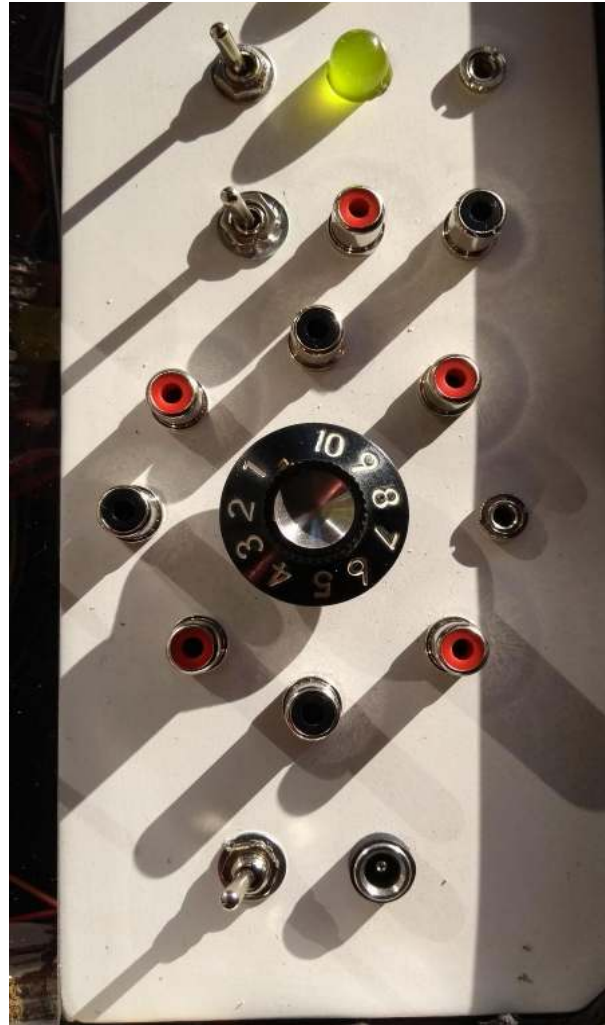
FIGURE 9: detail of bingo-splicer showing audio inputs and outputs (Photo: Author)
